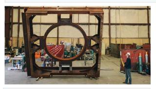
The Heavy Fabrication Department supports metal fabrication projects in material thicknesses of ¼" and greater and individual component weights in excess of 20 tons. This is accomplished in a variety of material types and to various industry fabrication standards. Our personnel possess the core skills to accomplish both routine fabrication as well as complex weldments requiring post-machining and critical non-destructive examination.
